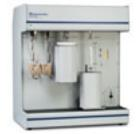
The ASAP 2020 Accelerated Surface Area and Porosimetry Analyzer
